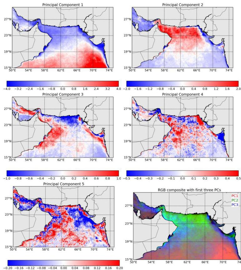
Figure R4 (Figure 2 from manuscript): Individual maps of principal components (PC 1 to 5) and RGB composite of the first three statistically significant components.
