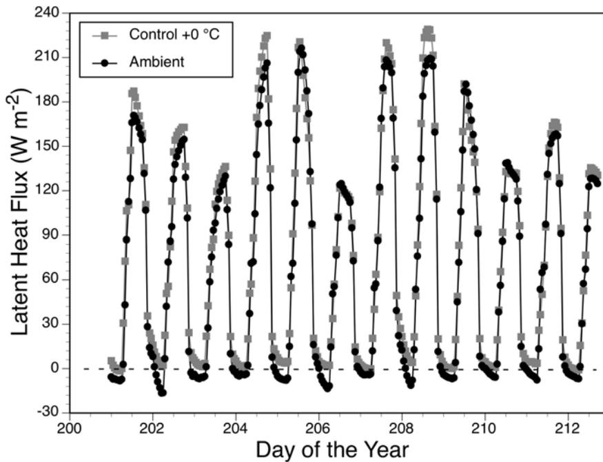
957 **Figure 16:** Simulations of latent heat flux over a 10-day period for ambient conditions (black)
