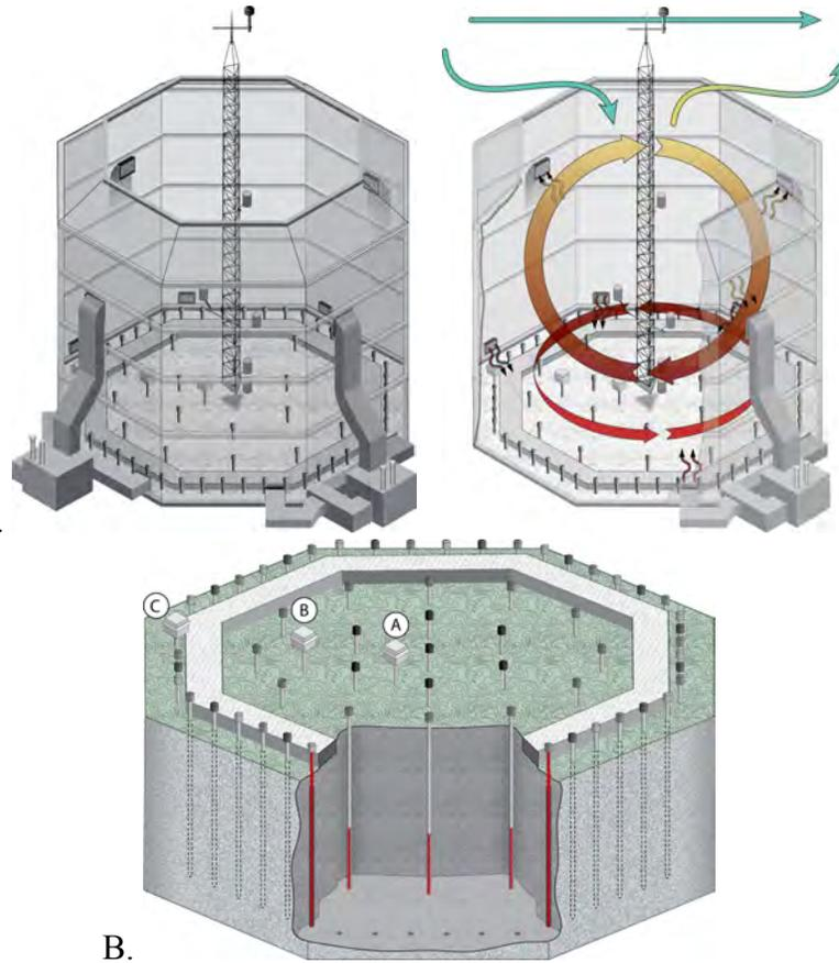
225 **Figure 2:** Panel A: Diagram of the air warming enclosure, warm air flow pattern, and external
