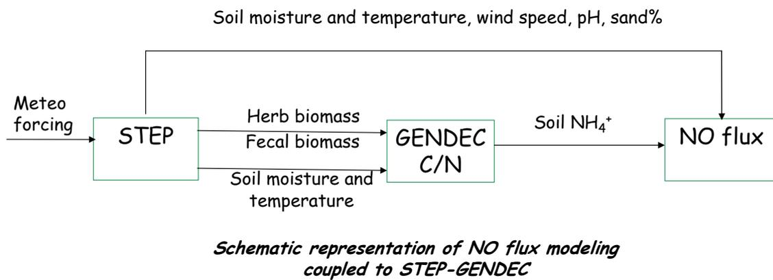
**Fig. 1.** Schematic view of links between the models STEP, GENDEC and NO emission model.
