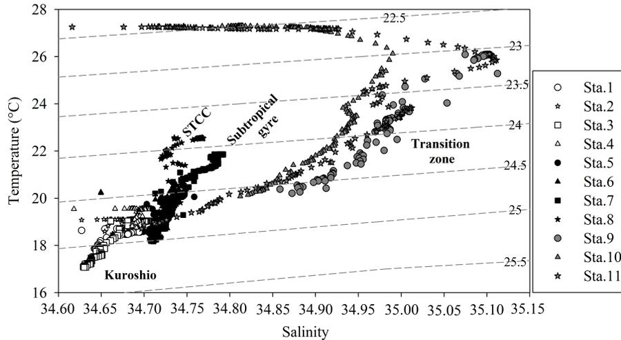
**Fig. 5.** Temperature-salinity diagram from surface to 200 m between stations 1 and 11. The three groups of stations are shown with different colors: stations in the Kuroshio region (1–4) by a white symbol; stations in the centre of the subtropical gyre (5–8) in black; and stations in the transition zone (9–11) in dark grey.
