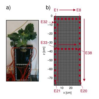
**Figure 1.** a) Experimental setup of plant root systems in water filled rhizotron. b) Corresponding finite-element grid used for electrical modeling and imaging. Red dots indicate position of electrodes.
