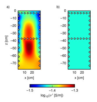
**Figure 2.** EIT inversion results (real component of complex conductivity) for measurements on a rhizotron filled with water of known conductivity (375  $\mu$ S/cm =  $10^{-1.43}$  S/cm) without (a) and with (b) correction of the impedance data for the imperfect 2D situation.
