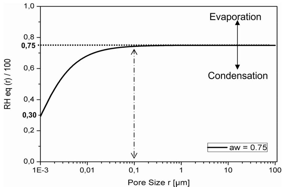
**Fig. 8.** Theoretical water evaporation/condensation equilibrium in halite. The model estimates the equilibrium relative humidity ( $RH_{eq}$ ) of a NaCl saturated solution as a function of pore radius (Benavente et al., 2003). See Supplement for more details.
