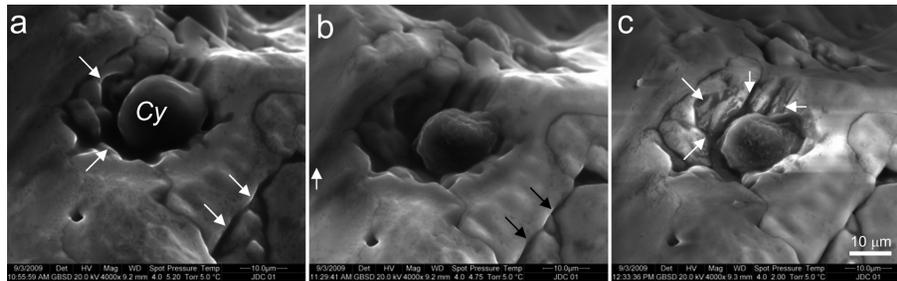
**Fig. 7.** ESEM in situ imaging of halite dehydration from RH = 76 % **(a)**; RH = 70 % **(b)**; and RH = 30 % **(c)**; Cy, cyanobacterial cells aggregate; white arrows point to brine solution; black arrows point to partially evaporated brine in narrow fissure. Note how the cyanobacterial aggregate shrinks with decreasing RH and brine evaporation. Scale bar applies to all images.
