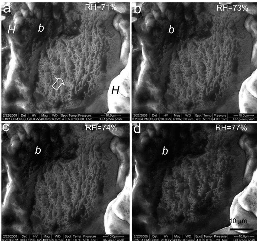
**Fig. 6.** Sequence of ESEM-BSE images showing the nano-porous phase (open arrow in **(a)** and central part of following images) among larger halite crystals (*H*) in samples equilibrated inside the ESEM chamber at RH between 71 % and 77 %; (*b*) = brine solution.
