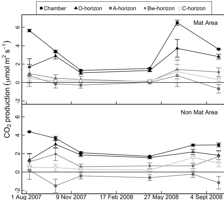
**Fig. 7.** Vertical partitioning of soil respiration over time. Measured surface CO<sub>2</sub> flux and calculated CO<sub>2</sub> production in the O, A, Bw1 + Bw2, and C horizons. Duplicate CO<sub>2</sub> profiles were combined and surface flux rates were averaged for each area. Error bars represent the propagated uncertainty from Monte Carlo simulations.
