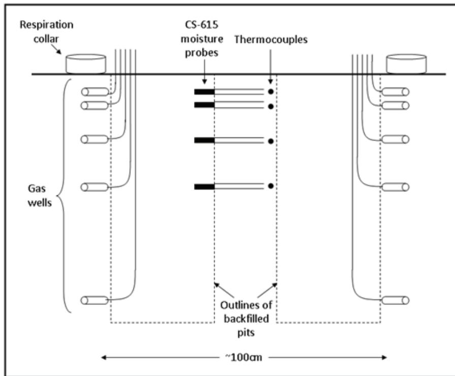
**Fig. 2.** Schematic of instrumentation used for vertically partitioning soil CO<sub>2</sub> production.
