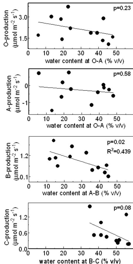
**Fig. 8.** Effect of soil moisture on production from each genetic soil horizon. Water content measured at the bottom of the O-horizon (top panel), and at the top of the other genetic soil horizons.
