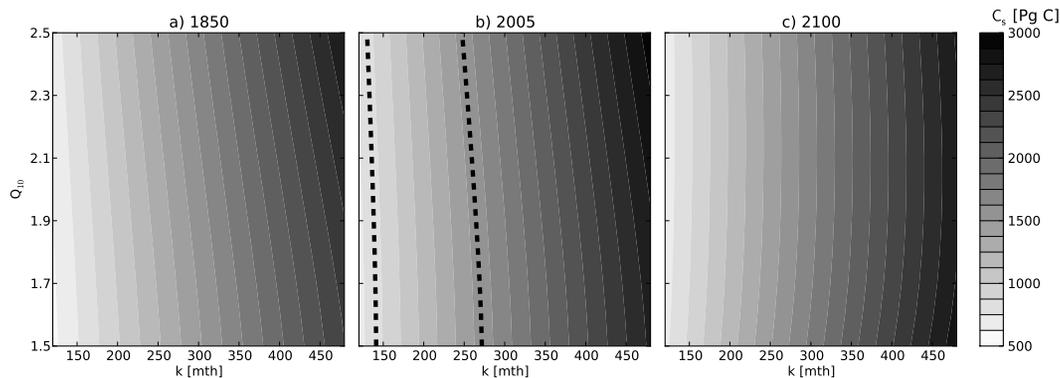
**Fig. 1.** Snapshots of total soil carbon in the reduced complexity model as a function of parameter values. Dashed contours in **(b)** indicate the  $CI_{95}$  of the HWSD in 2005 (830–1550 Pg C).
