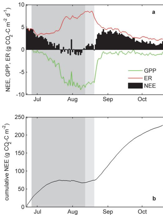
**Fig. 6.** Daily CO<sub>2</sub> budgets **(a)** and accumulated daily CO<sub>2</sub> fluxes **(b)**. Light and darker shaded areas represent the period between crop planting and harvest, and the period between harvest and disking.
